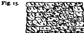
Fig. 15. Uncoursed or Random. —Beds and Joints undressed, projections knocked off, and laid at random. Interstices filled with spalls and mortar.
